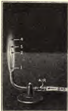
C. BUNSEN BURNER FLAME. HOLES ENTIRELY OPEN
